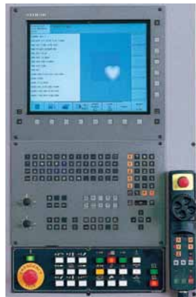
Heidenhain iTNC530 control
